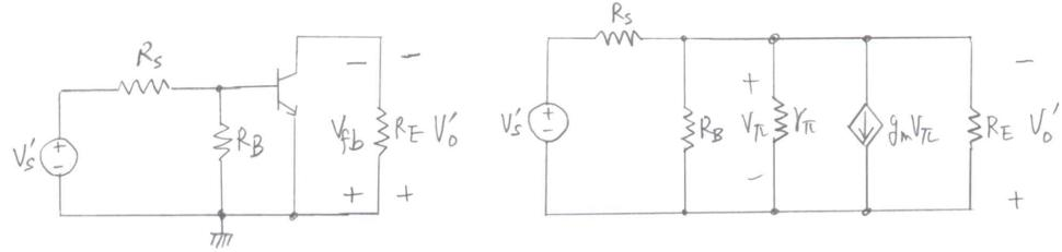
(b)  $A_v = \frac{(R_B \parallel r_\pi) g_m R_E}{R_S + (R_B \parallel r_\pi)}$
