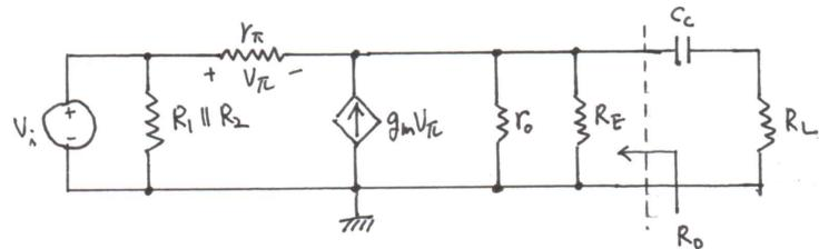
$$R_o = R_E \parallel r_o \parallel \left( \frac{r_\pi}{1 + \beta_o} \right)$$
